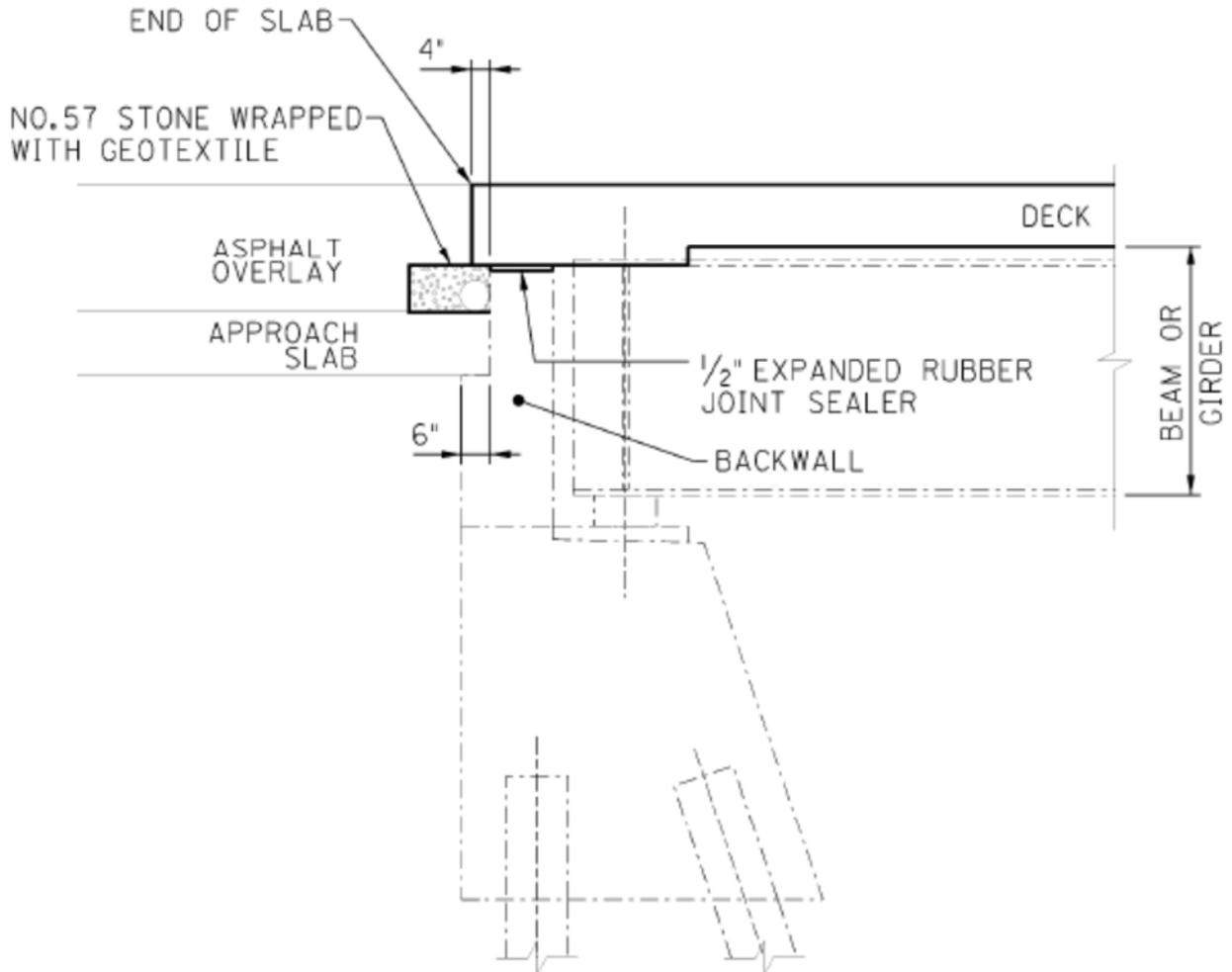
Figure 11: Abutment Joint Elimination by Slab Extension
