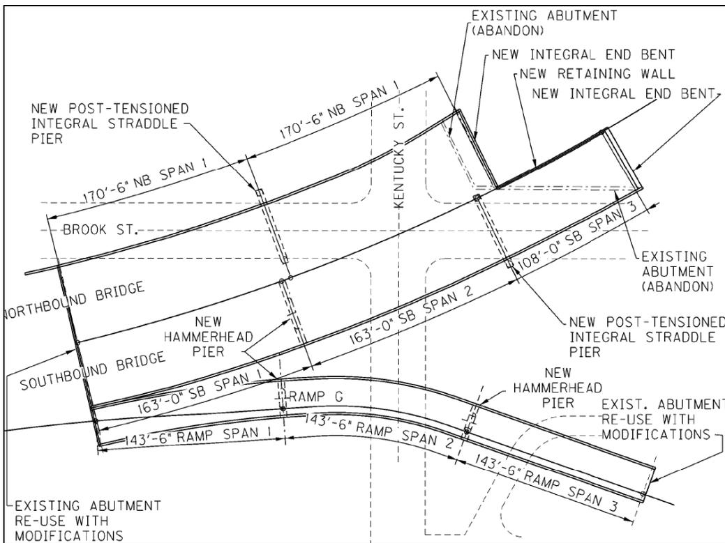
Figure 29: Bridge 183N Replacement – New Integral End Bents at South End
