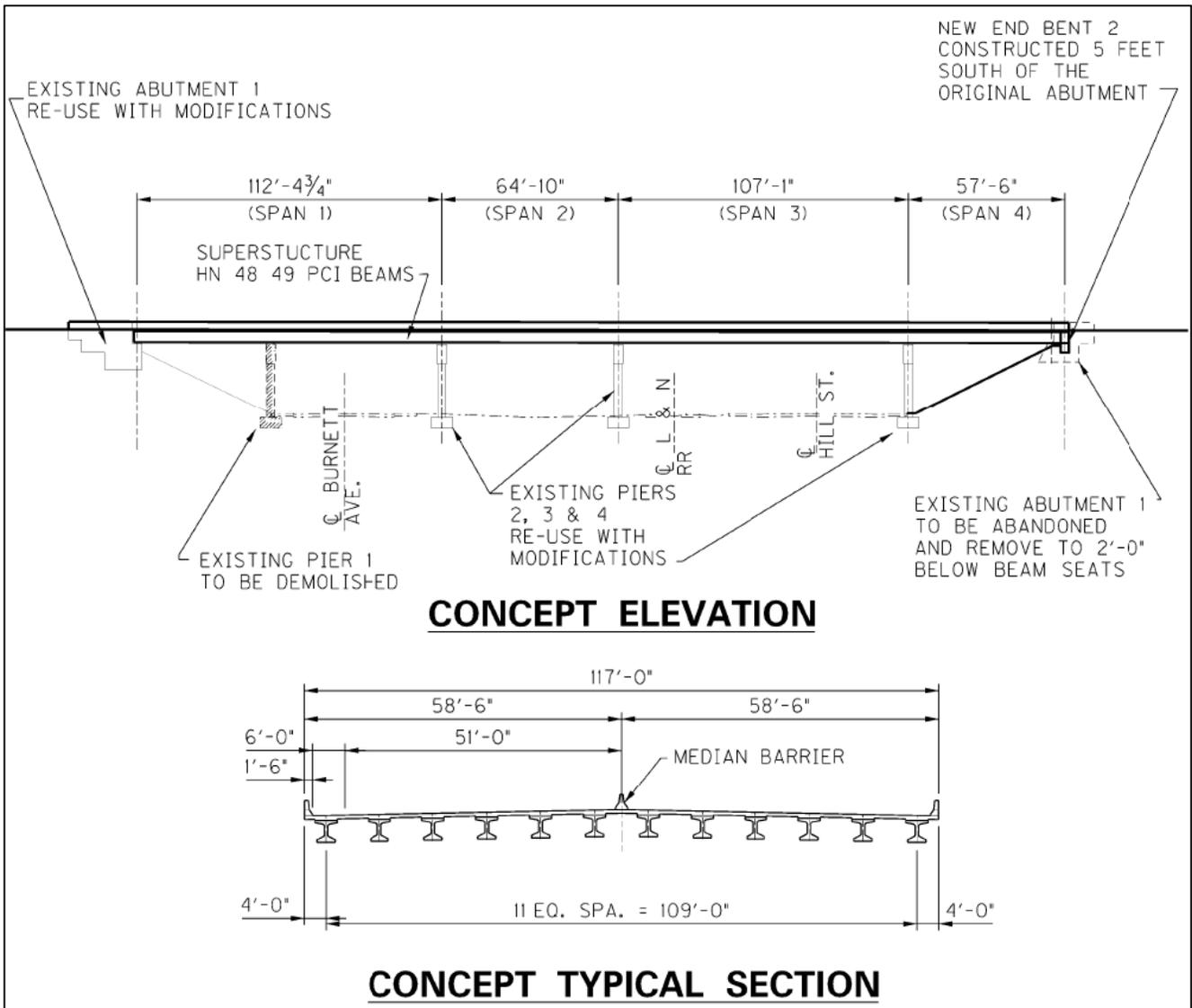
Figure 30: Bridge 179N Prestressed Concrete Girder Superstructure Replacement Option
