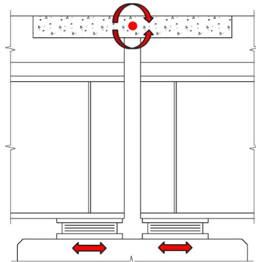
Pier Configuration with Link-Slab
