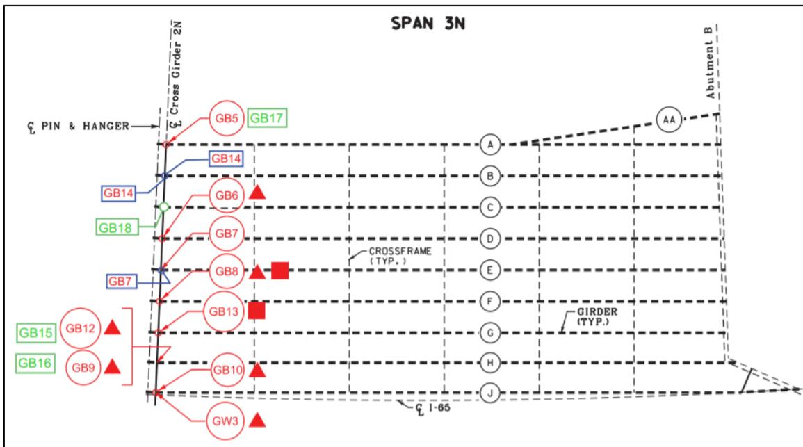
Figure 21b: Framing Plan (continued) Showing Crack Locations (2018 AECOM Bridge Inspection Report)
