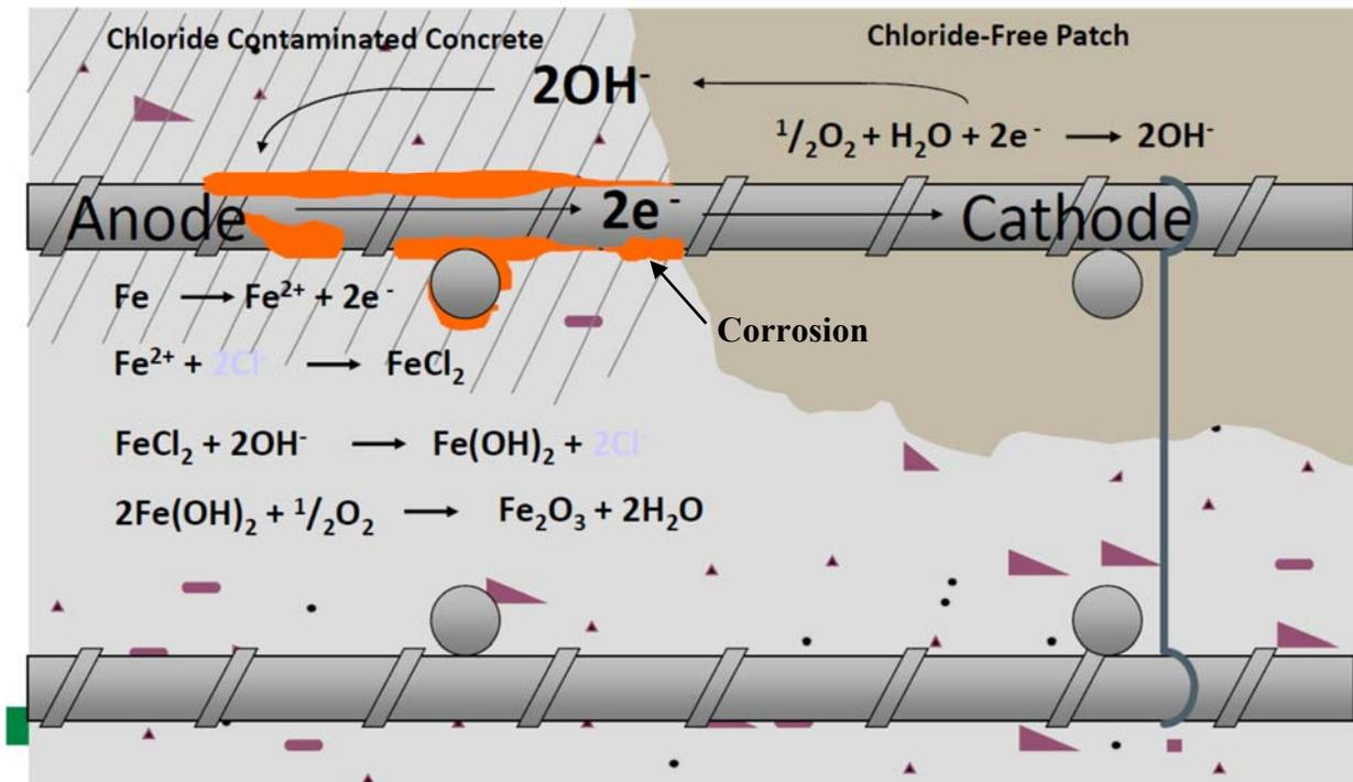
Figure 16: Conventional Patch Allows Corrosion to Continue (Vector Corrosion Technologies presentation)
