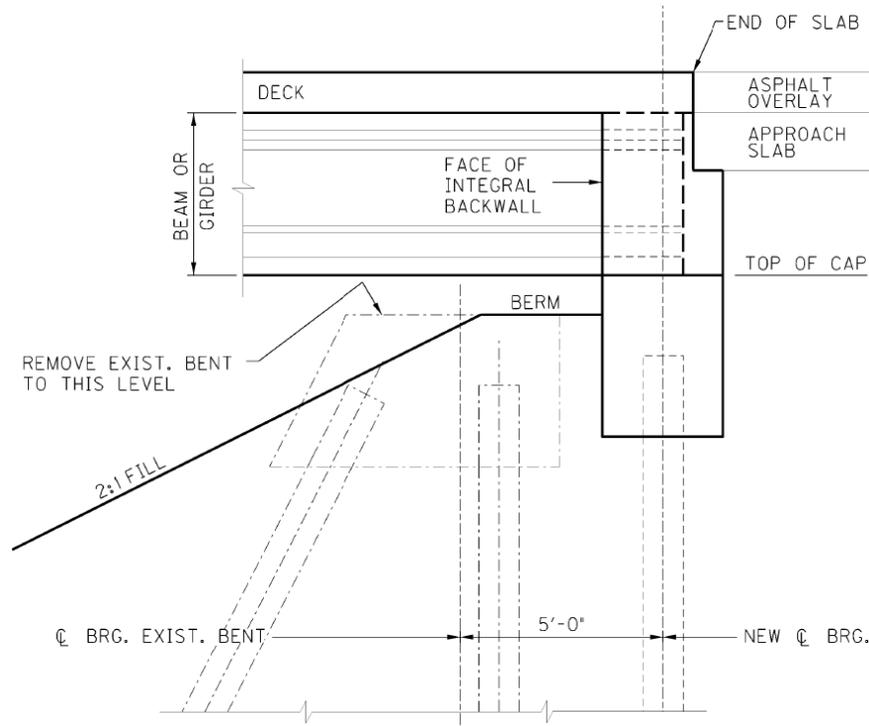
Figure 31: Bridge 179N - New Integral End Bents at South End
