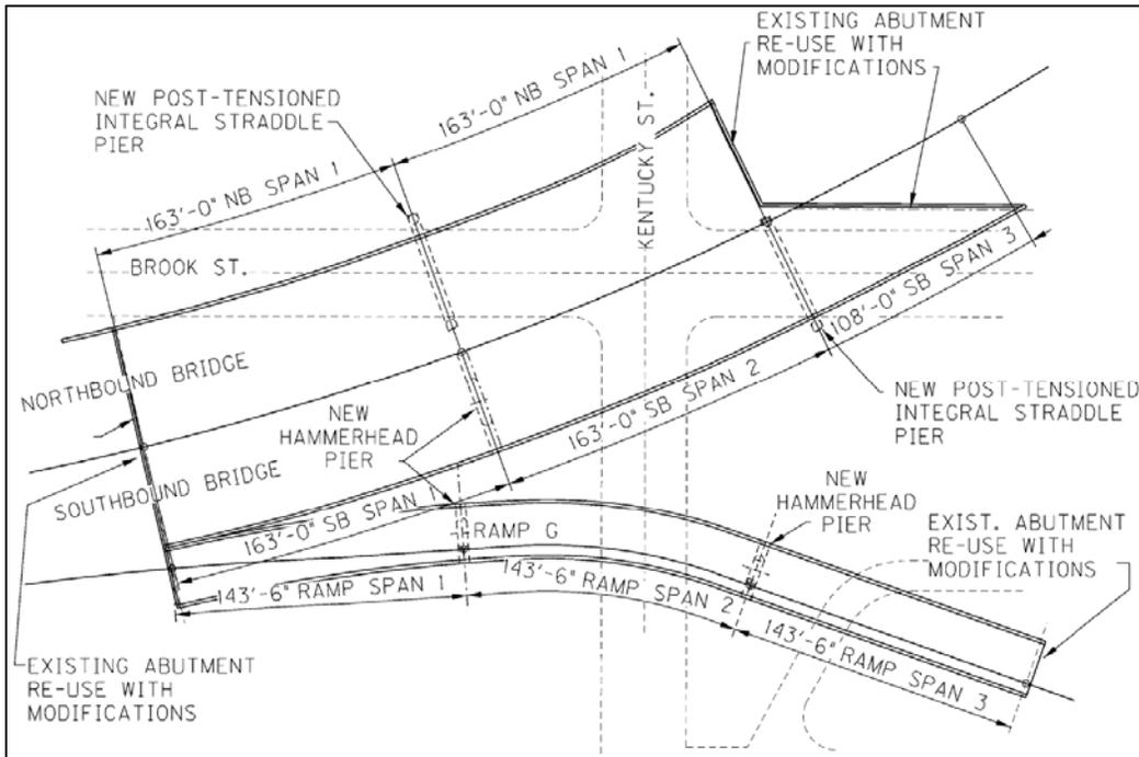
Figure 28: Bridge 183N Replacement – Reuse of Existing Abutments Option
