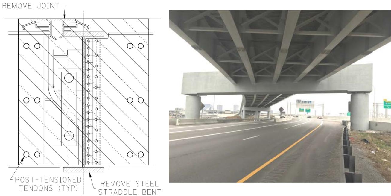
Figure 24: Post-Tensioned Integral Straddle Bent Option and Example from Kennedy Interchange
