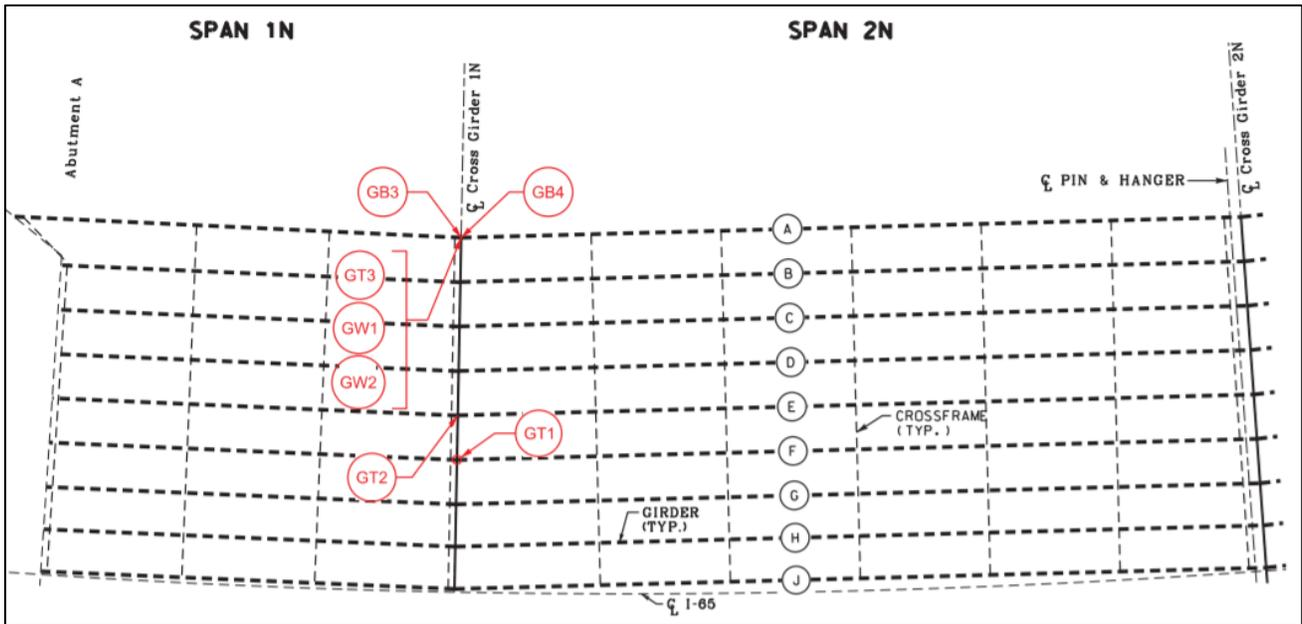
Figure 21a: Framing Plan (continued) Showing Crack Locations (2018 AECOM Bridge Inspection Report)
